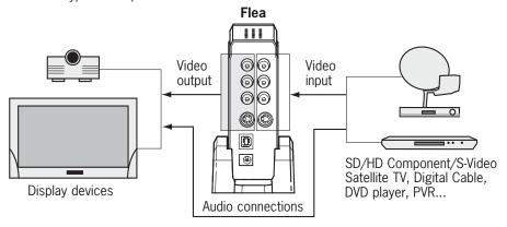
• **Flea** does not have audio processing capability. When two video sources are connected, switching from one source to the other will require external audio switching. The video processing delay introduced by **Flea** is negligible, and does not require any audio delay compensation.
